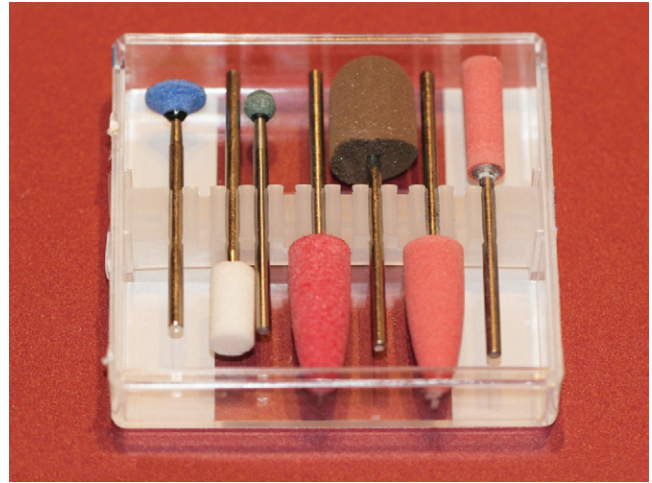
FIGURE 11-12 Kit for laboratory grinding and finishing of metals. Typically, green mounted stones contain silicon carbide and are useful for shaping, adjusting, finishing, and fine grinding of high-noble and noble cast alloys. The blue, brown, and white mounted stones are useful for noble and base metal alloys that are used for metal–ceramic prostheses. The pink mounted points and cylinder are used for hard metals such as cobalt–chromium alloys. The user should check whether these devices are intended for benchtop lathes or for handpieces.
