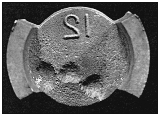
FIGURE 10-30 Surface irregularity on the cavity side of a casting caused by back-pressure porosity.
