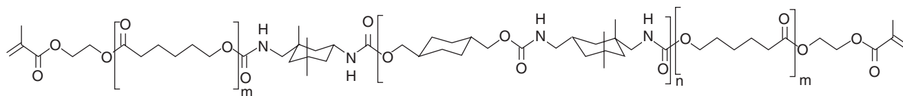
FIGURE 13-24 A high-molecular-weight polyurethane dimethacrylate monomer, DX-511, that contains a long, rigid central section between flexible methacrylate end groups ("Kalore," GC America, Alsip, IL). Like UDMA, DX-511 has urethane ( -\text{NH}-\text{CO}-\text{O}- ) groups that connect a central segment between two ethylmethacrylate end groups. It also contains 2m + 1 cyclohexane rings. (Courtesy of Barry K. Norling.)
