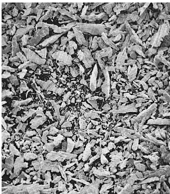
FIGURE 15-1 Particles of conventional lathe-cut alloy for dental amalgam ( \times 100 ).
