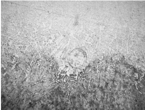
FIGURE 16-5 Micrograph showing alloying at the interface between a gold-alloy solder metal and a base metal substrate (×100). (Courtesy of C. E. Ingersoll.)
