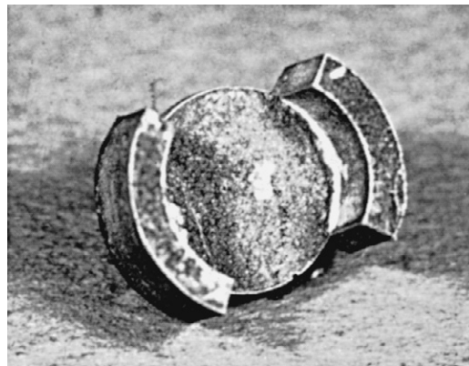
FIGURE 10-27 A black-coated noble metal alloy casting resulting from sulfur contamination or oxidation during melting of the alloy.
